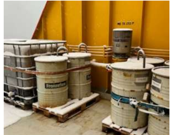
New "goose neck" vents on waste containers (post-event)
