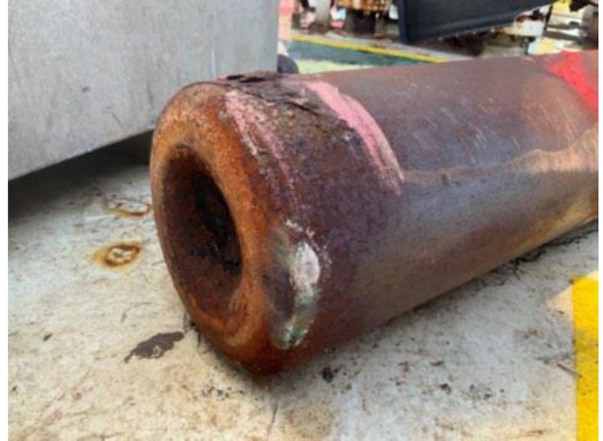
Base of bottle showing corrosion
