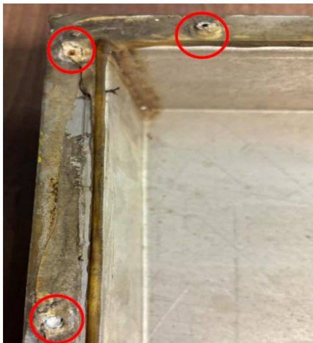
Failed aluminium rivets
